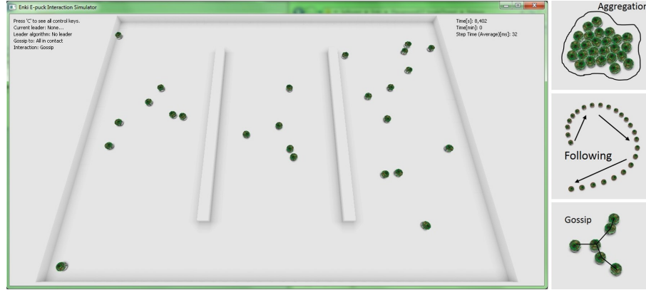
Fig. 1: Snapshot showing the simulation environment from a bird’s-eye perspective. The operator is not provided with this global state information (except for the control experiments). The robots can perform three swarm behaviors: aggregation (top right), following (middle right), and gossip (bottom right).
