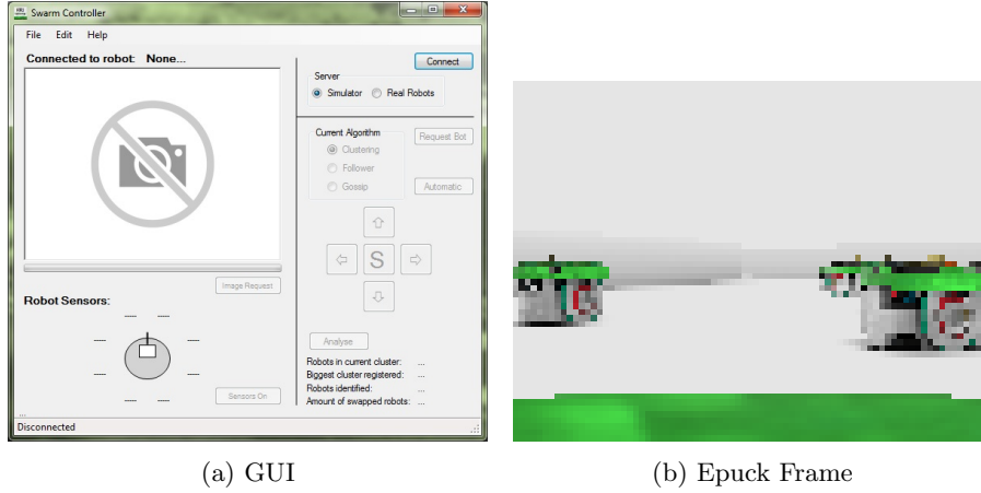
Fig. 2: (a) Graphical user interface that the participants used in the human-robot swarm interaction study. (b) Image taken by a simulated robot and provided to the operator via the graphical user interface.
